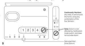
open, storage sheds or work shops unsecured, etc). Sensors placed in Zone 4 will not activate the Alarm or Chime. When a Sensor is triggered in Zone 4, the Control Center will sound a repeating Alert (4 beeps) and the Zone 4 LED indicator will flash continuously. These Alerts will continue until the Sensor is closed. You can Mute the repeating Alert sound but the LED indicator will continue to flash until the Sensor is reset/deactivated (i.e. door is closed).
